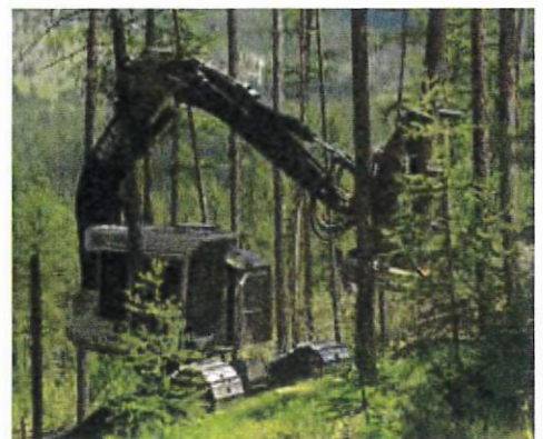
Directional falling and/or reaching into the SMZ with a mechanical feller-buncher allows removal of some SMZ trees without damaging the SMZ.
