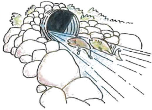
Water may be too shallow for fish to swim. This is sometimes a problem created by squash pipes that are used when road clearance over the pipe is limited. Shallow water leaves fish partially submerged and unable to get maximum thrust from tail and body movements.
