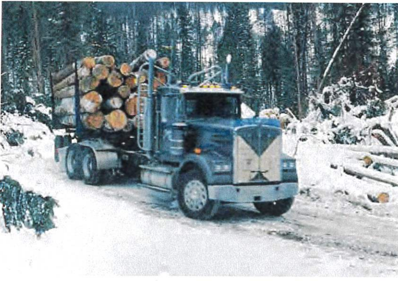
To provide a winter road grade capable of heavy hauling, always remove snow cover. Deep-frozen road surfaces have tremendous strength. Do not let snow cover insulate and weaken the road—plow during cold weather.
